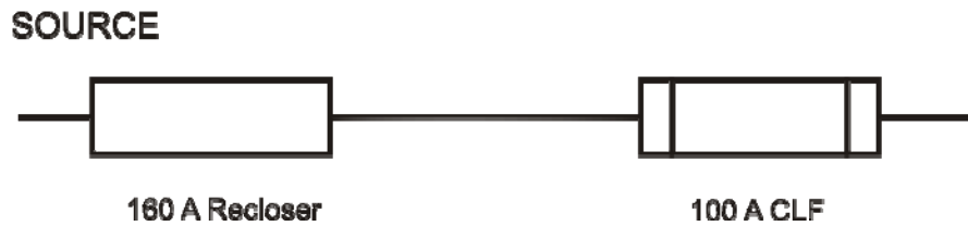
Figure 16—Recloser/Current-limiting fuse example
