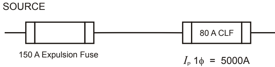
Figure 14—Expulsion fuse/Current-limiting fuse example
